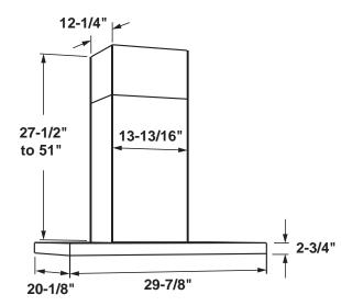
30"models require a 30"-wide opening \*The supplied duct cover fits 7'-7" to 10'-6" ceiling heights (12' ceiling height with optional high celling kit UX12DC9SLSS/UX12DCBLTS) (14' ceiling height with optional high celling kit UX14DC9SLSS/UX14DC9BLTS)
