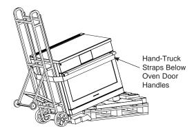
6. Move the range indoors. Position the range in front of the installation location.
