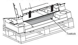
Drive the blade of the hand-truck beneath the foam block.
