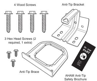
Attach the anti-tip brace onto the bottom of the range in the recessed area. Install 2 hex screws (provided) through the brace and into the range.
