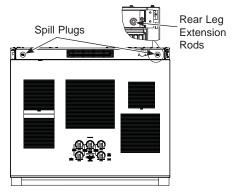
Do not adjust legs over the 36 15/16" maximum unit height (as specified on Pages 4-6) with respect to whatever surface the range sits on.
