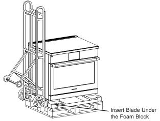
**IMPORTANT:** Do not remove the base foam block while the hand-truck is in use. Place the hand-truck blade underneath the base foam block and transport the range to the final location.
