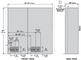
DUAL INSTALLATION 30" INTEGRATED FREEZER, ZIF301NPNII AND 30" INTEGRATED REFRIGERATOR, ZIR301NPNII
